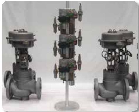
Pipeline control valves with detached control blocks
